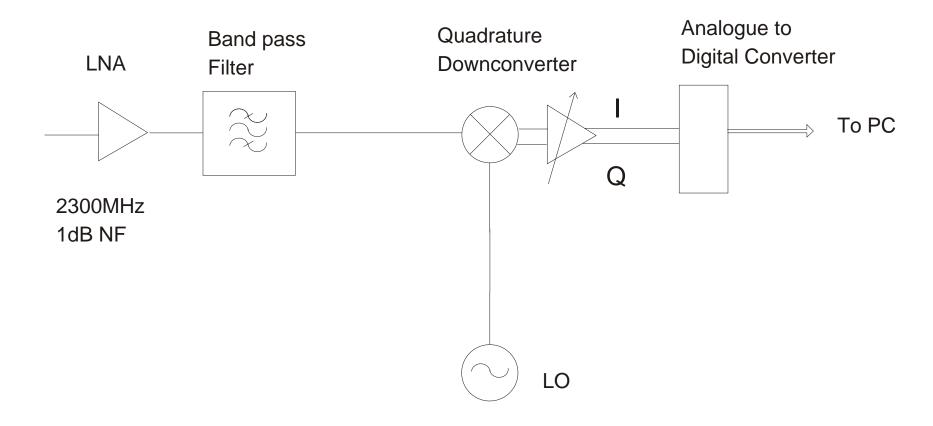
Low-noise amplifier, band-pass filter and Local Oscillator all operate from 2300-2450MHz.
